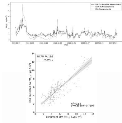
Top: Time series of PM<sub>2.5</sub> observations from the Longmont EPA instrument (green), the raw data from the collocated NCAR PA1& PA2 monitors (orange), and the EPA corrected data for the NCAR PA1& PA2 monitors (black) during a 2-week time period in June 2022.
