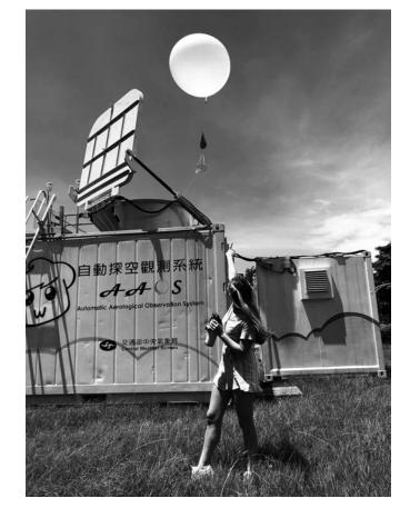
Taiwan's Central Weather Bureau (CWB) Automatic Radiosonde Launcher. Radiosondes launched at 00 UTC, 06 UTC, 12 UTC, and 18 UTC for the PRECIP field campaign. Source: Angelie Nieves Jiménez at Hsinchu, Taiwan (PRECIP 2022)
