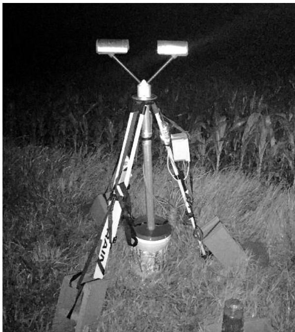
The deployment of an Ott Parsivel optical laser disdrometer in a field ahead of an MCS in northeastern Kansas.
